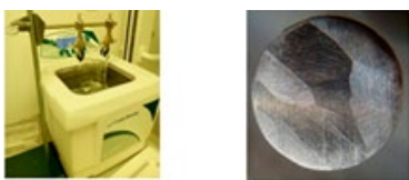
FIGURE 1. Ultrasonic bath and morphological surface of washed Mg before the phosphate treatment.
