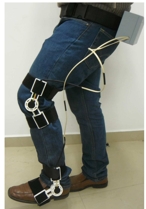
FIGURE 1. The ELLTIO prototype with two degrees of freedom and the motion capture prototype for knee and ankle.
