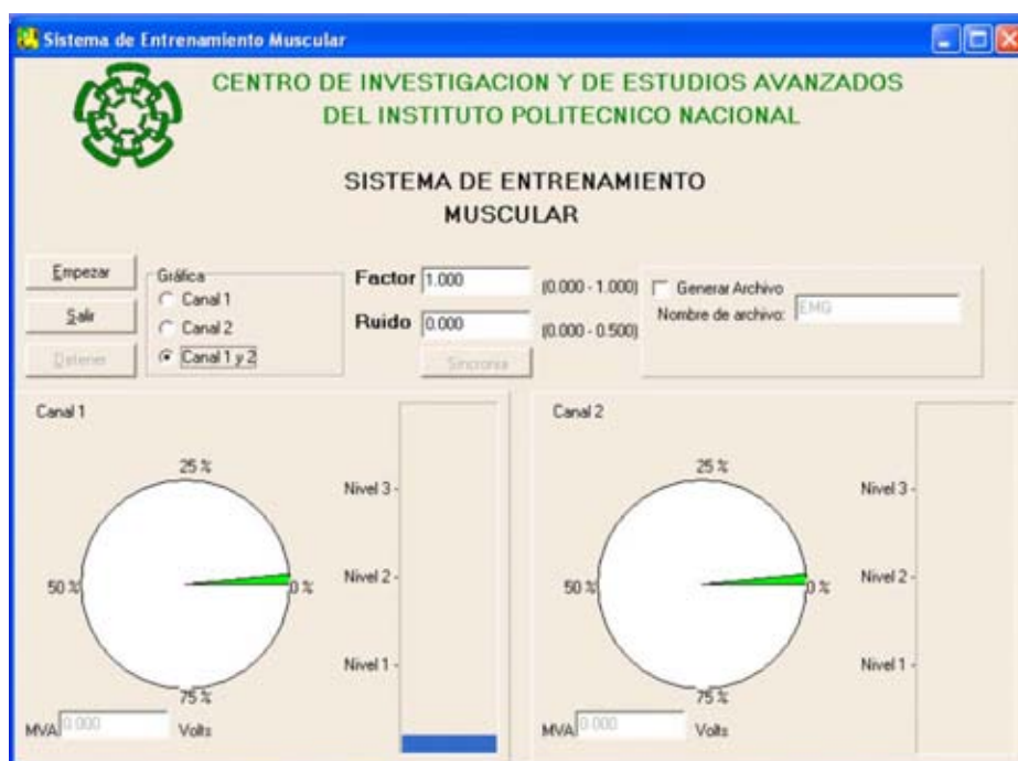
Figure 2. Myoelectric trainer. Muscular activity of each user is showed by mean of graphics.
