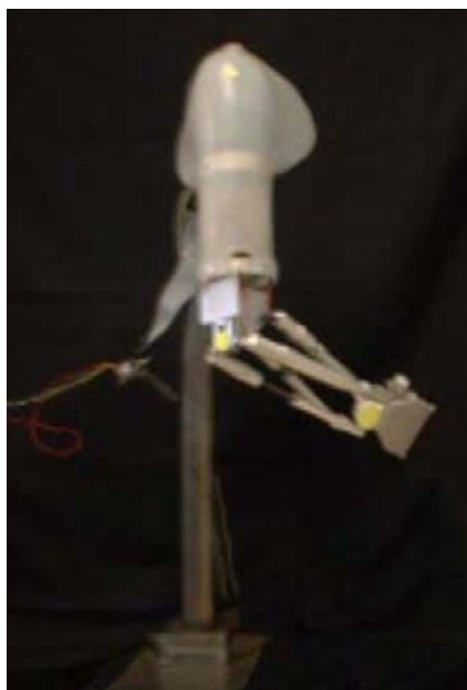
Figure 3. CINVESTAV-IPN Prosthesis prototyped mounted on a pedestal and controlled by a RS-232 interface.
