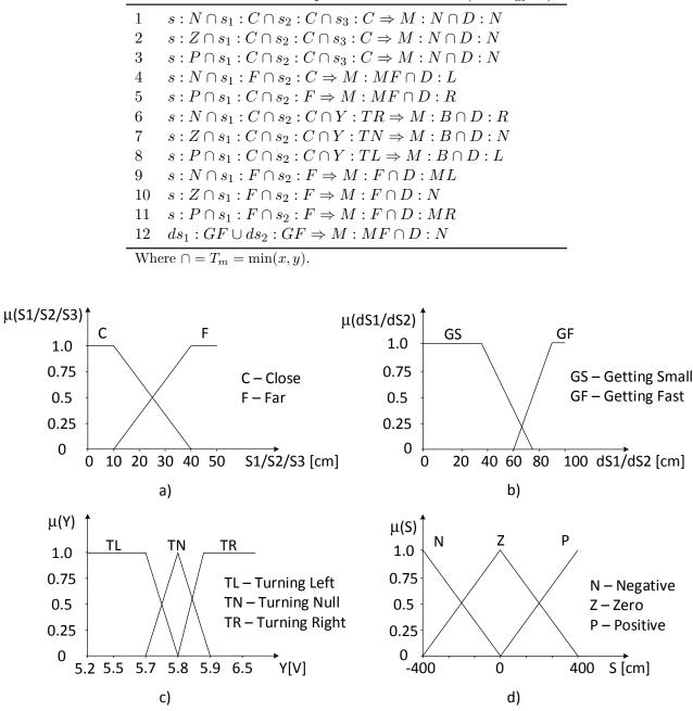
Figure 6. Fuzzy Input definitions and memberships functions a) distance, b) distance differential, c) past steering action and d) sensor difference.
