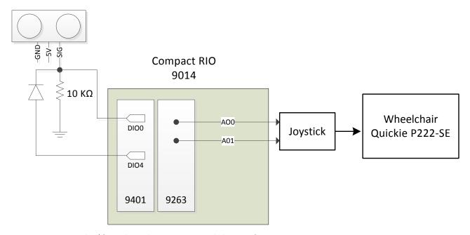
Figure 12. Digital I/O and analog output modules configuration.
