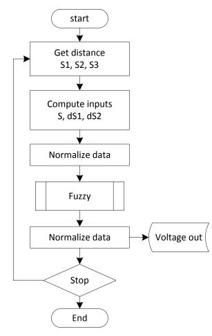
Figure 16. *fuzzy logic* controller block diagram
