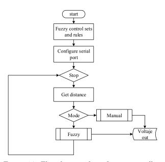
Figure 14. Flux diagram for software controller implementation.
