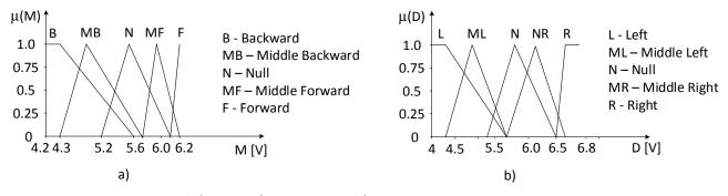
Figure 7. Fuzzy outputs definition a) Movement, b) Direction outputs
