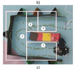
Figure 20. Obtained trajectories in test scenario. Dots represent lateral sensor position during the route, a) Strategy A, b) Strategy B, c) Strategy C.
