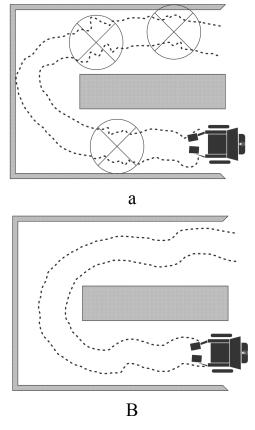
Figure 21. Hardware and software trajectory tracking comparison for the Strategy-C using, a) Computer device b) Compact-RIO.
