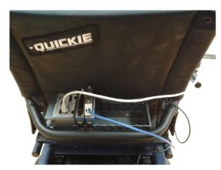
Figure 18. NI Compact-RIO installed for the real-time system.
