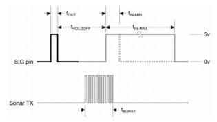
Figure 3. Figure 3. Parallax PING))) ultrasonic sensors principle of operation described in their manual [33].
