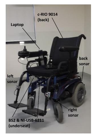
Figure 19. The complete system. For the hardware implementation, the laptop is only used for setting the controller initial conditions and to register data.
