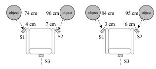
Figure 8. Case Study regarding the configuration when both sensors change values (a) at same speed and (b) S1 changes faster than S2.
