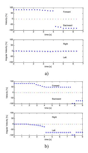
Figure 10. The velocity graphs for configurations (a) obstacles moving at the same speed (b) obstacles moving at different speed.
